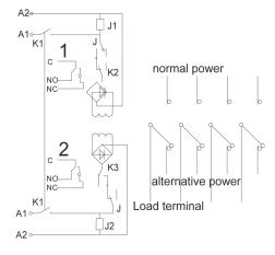
K1:Manual/Electric selection switch K2、K3:Product internal position seitch J1:Power A 220V relay J2:Power B 220V relay 1:Power A passive signal output 2:Power B passive signal output
